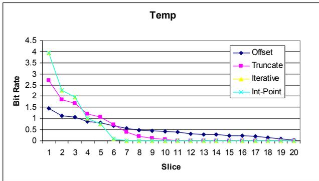
Figure 6. Bit allocation for NOGAPS temperature
